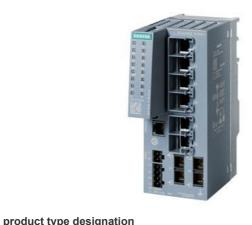
SCALANCE XC206-2 managed Layer 2 IE switch; IEC 62443-4-2 certified; 6x 10/100 Mbps RJ45 ports; 2x 100 Mbps SC ports; 1x console port; diagnostics LED; redundant power supply; temp. range -40 °C to +70 °C; mounting: DIN rail/S7 mounting rail/wall; redundancy functions; Office features (RSTP, VLAN,...); PROFINET IO device Ethernet/IP-compliant C-plug slot
